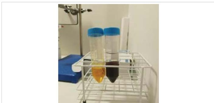
Figure 3: Vegetable oil sample, before and after acid-silica (55 %) cleans up.
