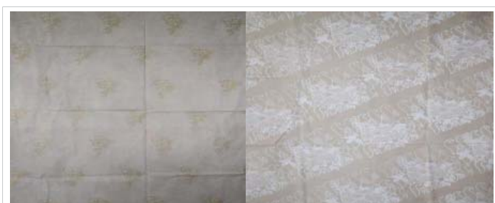
Figure 5: Application of colors mixture at prmissima fabrics ( C. Sappan , R. mucronata + X. granatum ) leaves, visual color, fixation lime. Fabric immersion: 7 times in aqueous of extract, and color ultimately appeared: greenish brick-red.
