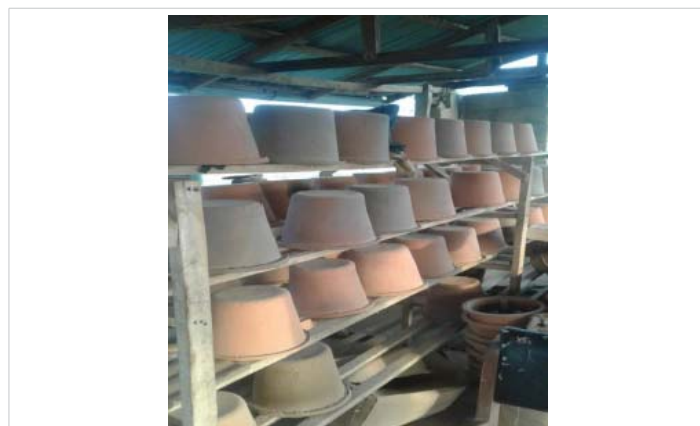
Figure 6: Sun-drying of ceramic filters.
