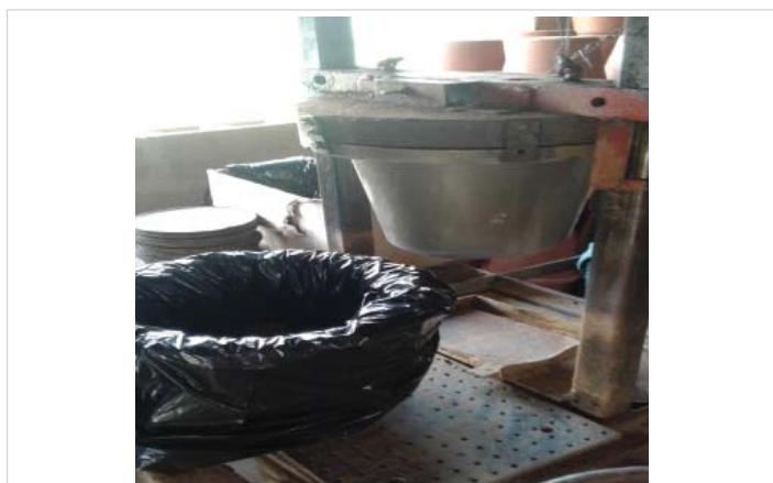
Figure 5: Molding press for the ceramic filter.
