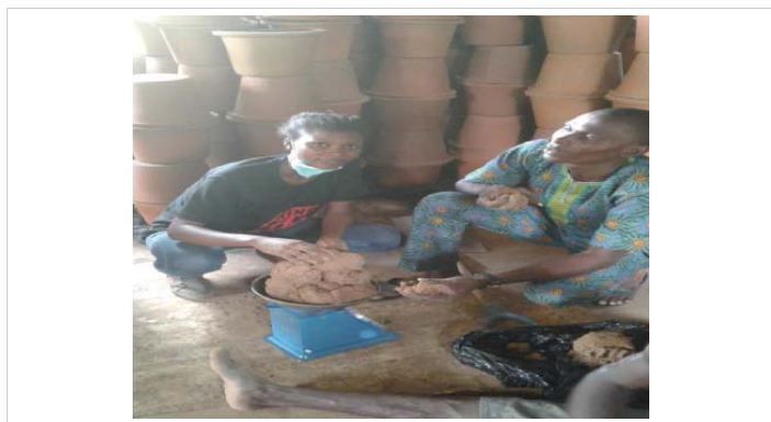
Figure 4: Weighing of the clay-sawdust matrix before molding.
