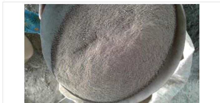
Figure 2: Pulverised and sieved clay sample.
