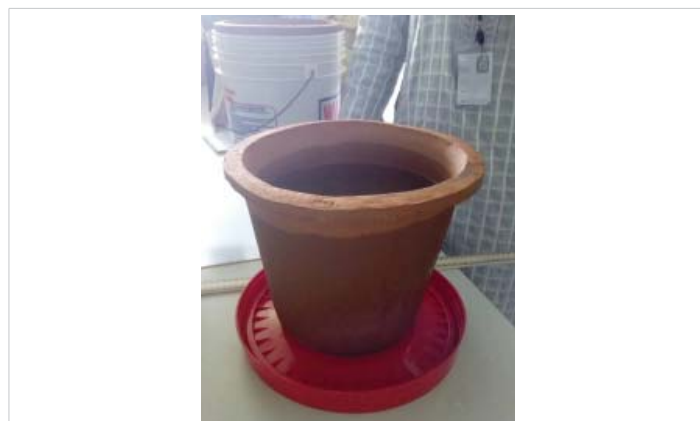
Figure 7: Water saturated ceramic filter just before filtration.
